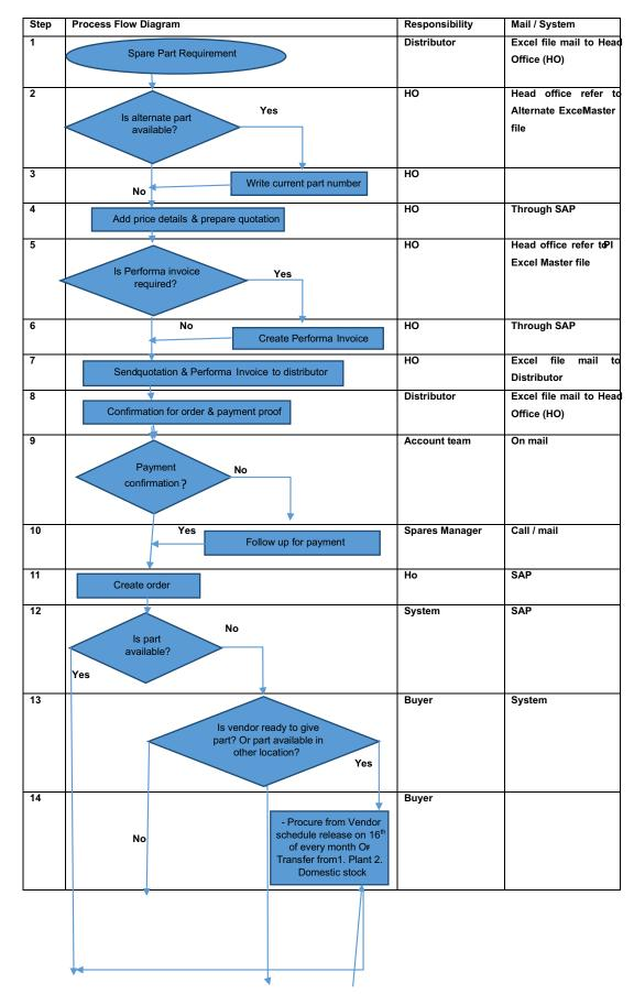
Step by step process of part requirement to dispatch (Before improvement made). Table 1
